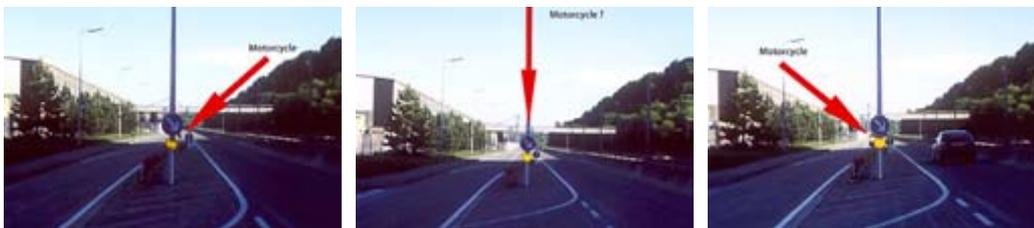
Positioning and construction of **road signs**, lighting standards and other road furniture must include the safety needs of motorcyclists.
