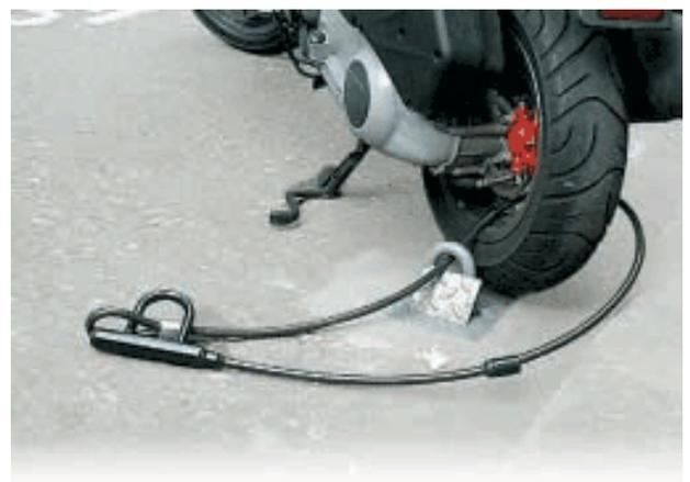
Example of a ground level locking system
