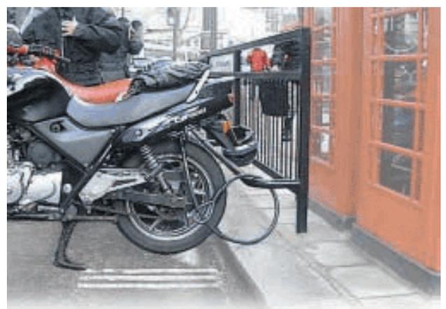
Example of a raised (horizontal bar) locking system
